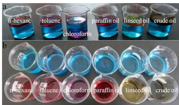
Figure 4. Photographs of (a) before and (b) after separating oil/water mixtures. [Color figure can be viewed in the online issue, which is available at wileyonlinelibrary.com.]
